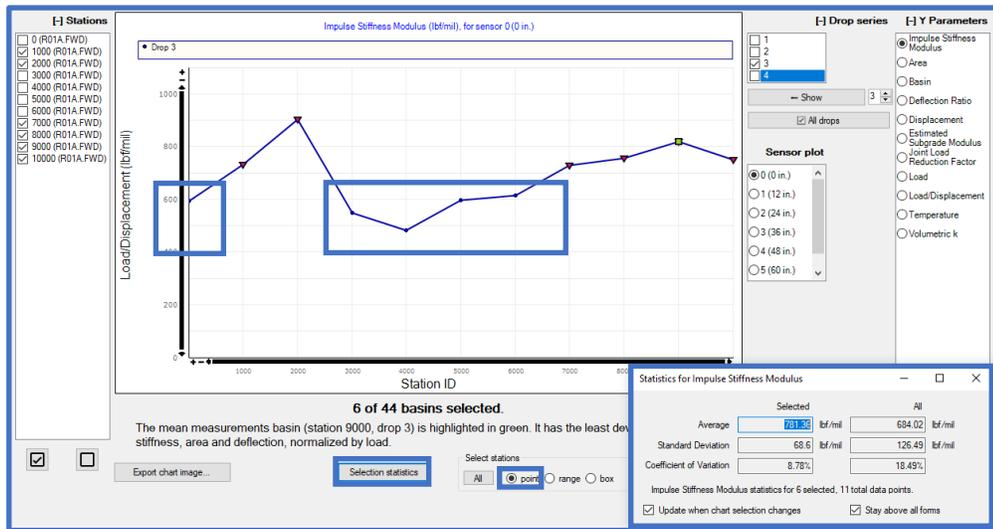
Step 9. Jane then toggles to the **Basin Y Parameters** to view the respective **Deflection Basins**. She observes that the deflection basins for these five stations with low ISM values exhibit higher displacement values for D1 when compared to the other stations. The displacement values for D2-D7 seem to be fairly consistent across all the stations.
